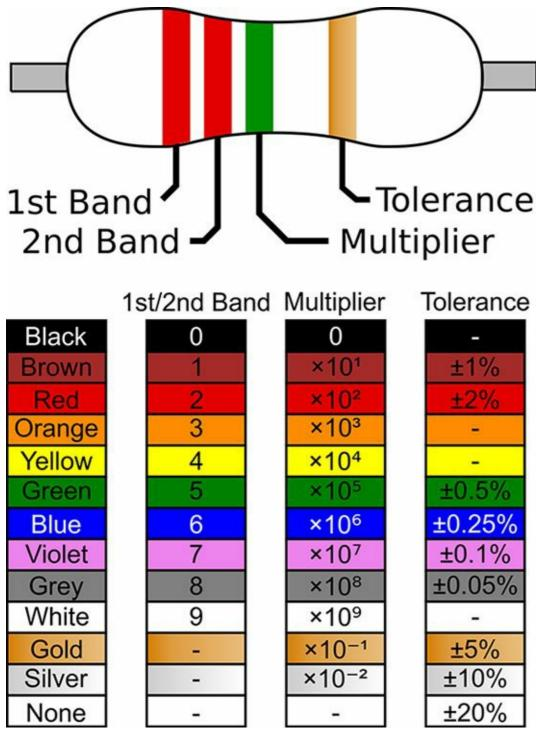
To read the example resistor, first take the two resistance bands starting from the left: these are coloured red and red. Red, on the table included in Figure 12-1, equates to the value 2, so the initial reading is 22. The next band is green, which is the multiplier and equates to 105 or 100,000 (10 followed by five zeros). Multiplying 22 by 100,000 equals 2,200,000, which is the resistance value in ohms: 2,200,000  $\Omega$ .
