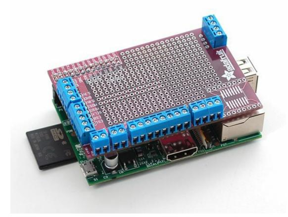
The design and layout of the Prototyping Pi Plate will be familiar to anyone who has used an Arduino microcontroller. An add-on board with the same footprint as the target device, designed to connect to on-board headers and sit above the surface of the original board is a common sight in the Arduino world, where such add-on boards are known as shields. The idea for the Prototyping Pi Plate, in fact, comes from Adafruit's self-designed Protoshield add-on for the Arduino.
