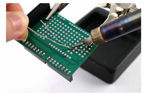
**4.** As the solder flows, you'll see it drawn down into the hole in the board. This is an indication that the area is hot enough for a good solder join. If the solder floats, it indicates that the area is not yet hot enough.
