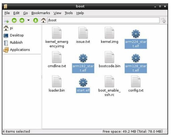
The first file, arm128\_start.elf, is configured to split the memory down the middle, with 128 MB available to the BCM2835's ARM CPU and 128 MB available to the VideoCore IV GPU.
