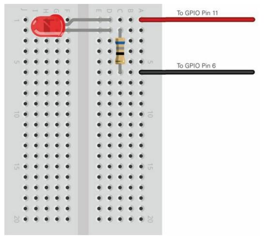
At this point, nothing will happen. That's perfectly normal: by default, the Raspberry Pi's GPIO pins are switched off. If you want to check your circuit immediately, move the wire from Pin 11 to Pin 1 to make the LED light up. Be careful not to connect it to Pin 2, though: a current-limiting resistor suitable for a 3.3 V power supply will be inadequate to protect the LED when connected to 5 V. Remember to move the wire back to Pin 11 before continuing.
