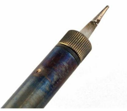
This process of tinning the tip protects it against damage and ensures that it will efficiently transfer heat onto the surfaces to be soldered. Failure to properly tin the iron's tip is one of the most common causes of bad solder joints. You may need to repeat this process more than once if you're soldering a lot of connections, and you'll need to do it again at the end of the soldering session. In general, if the tip of the soldering iron loses its shiny coating, repeat the tinning process.
