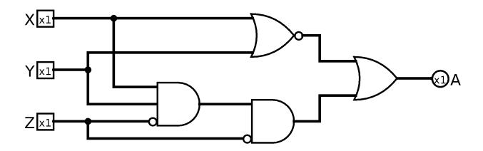
First, write the Boolean expression corresponding to this circuit. (Don't worry about the "x1". It indicates that the connection is for a single bit.)
