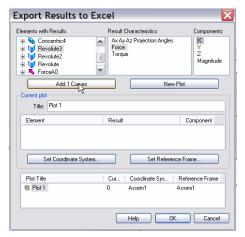
We will plot both components of force (the Z-direction force is zero) and the magnitude on a single graph.
