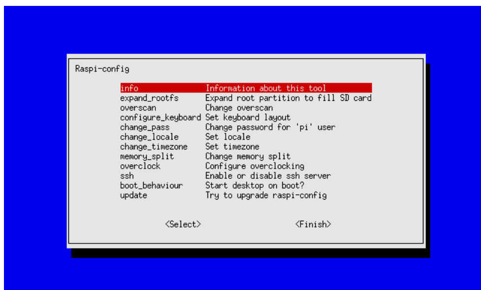
Figure 1.9 The Raspberry Pi config tool. The highlight bar can be moved between the different controls using the Tab key, or up and down in the menu using cursor keys.
