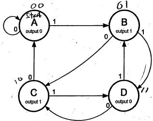
1. Suppose the FSM is started (in state A) and then receives three successive inputs 0 1 1. After the 3<sup>rd</sup> input bit is received, which state is the FSM in and what is its output?
