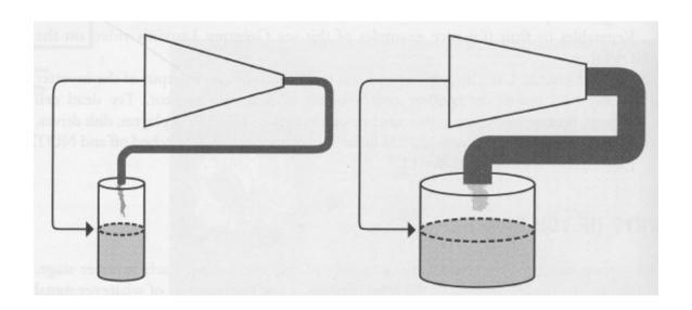
The capacitor discharges and sends its liquid contents to the funnel when the liquid reaches the dotted line. The discharge is the clock tick. Once the glass is empty, it is refilled by the pipe. Together the size of the glass and the size of the pipe determine the rate at which the clock ticks. The slowest clock has the biggest glass and the smallest pipe.
