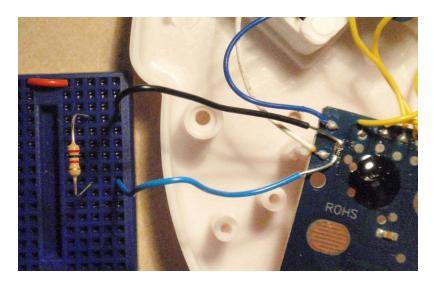
A breadboard allows you to make electrical connections without soldering which is something you can now appreciate. Breadboards are used for prototype development-they are "clunky" but very easy to change. Electrical connections (pathways for current to travel) are built into a bread-board as described <a href="here">here</a>.
